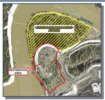
White contour lines in the figure above show the approximately 30-foot tall pile of steel "slag" that was removed during the project. After removal, the project area was restored to natural floodplain. With time, it is anticipated that the restored area will mimic habitat conditions present in the existing heron rookery.
