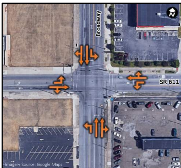
Figure 4: Broadway Intersection Lane Configuration
