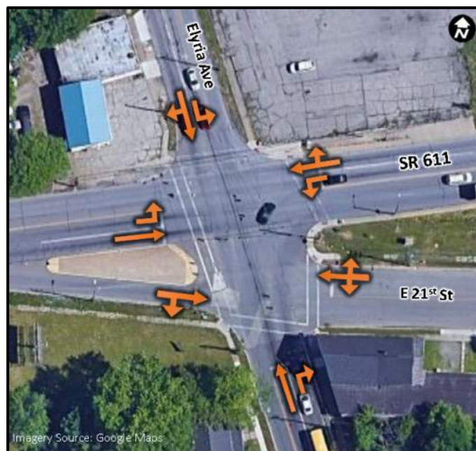
Figure 17: SR 611 and Elyria Avenue Roadway Reconfiguration Lane Configuration
