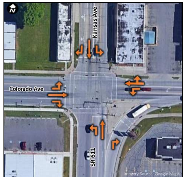
Figure 16: SR 611 and Colorado Avenue Roadway Reconfiguration Lane Configuration
