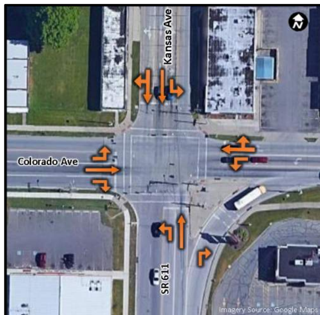
Figure 2: Kansas Avenue/Colorado Avenue Intersection Lane Configuration
