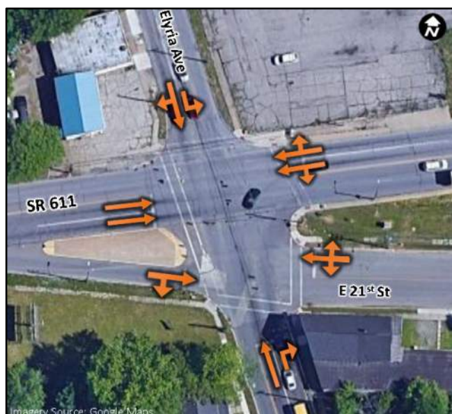
Figure 3: Elyria Avenue and E 21 st Street Intersection Lane Configuration
